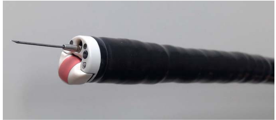
► Fig. 2 Photograph of the forward-viewing echoendoscope (TGF-UC260J, EU-ME1; Olympus Medical Systems, Tokyo, Japan).
