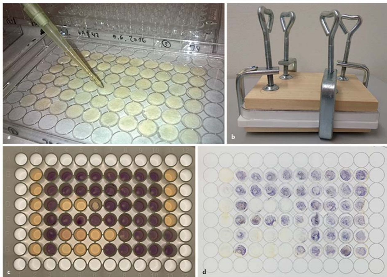
► Fig. 6 Microdilution volatilization method [65] (original author's photos). a Agar pipetting into every flange on the lid. b Use of clamps for fastening plate and lid together. c Colouring of the living bacterial colony with MTT in the plate (broth culture). d Colouring of the living bacterial colony with MTT on the lid (agar culture).
