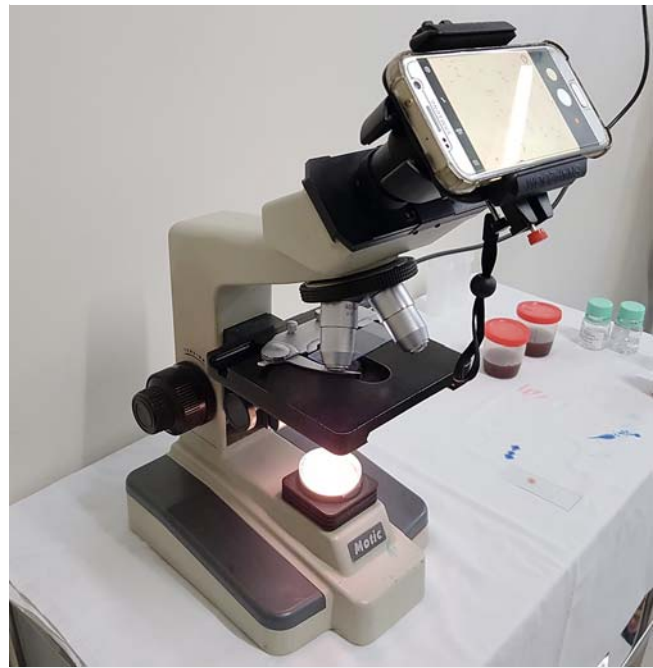
► Fig. 1 Microscope fitted with an Android smartphone for smear evaluation and image capture.
