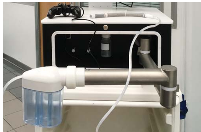
► Fig. 2 The robotic colonoscope: the workstation with the probe attached.
