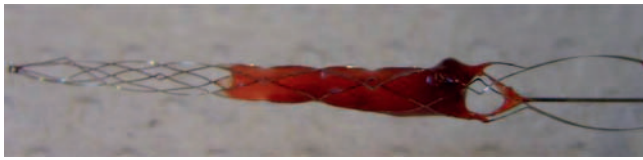
► Fig. 1 Prototyp I (40 \mu m stent struts, tapered design, 2,0 – 3,5 \times 35 mm) with thrombus.
