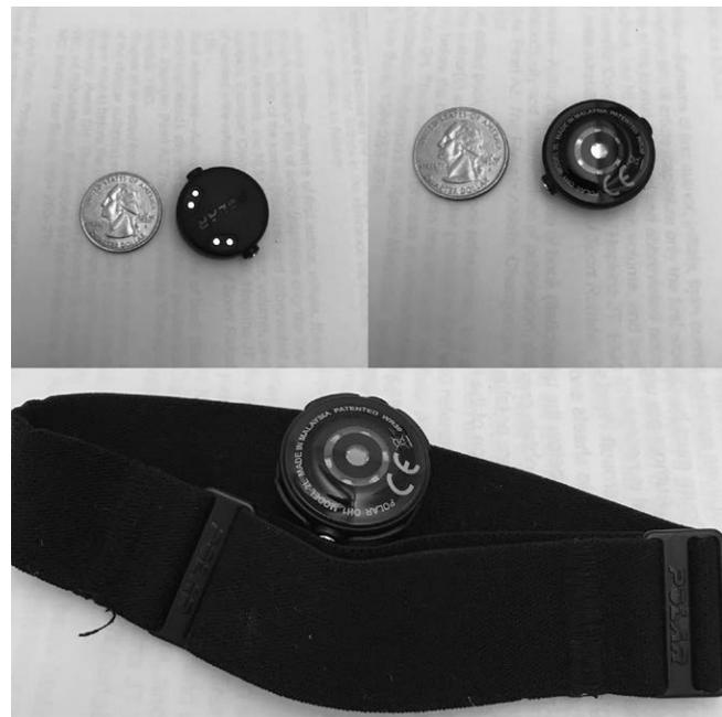
► Fig. 1 Polar® OH1 optical arm-band heart rate sensor. US quarter-dollar shown for scale.
