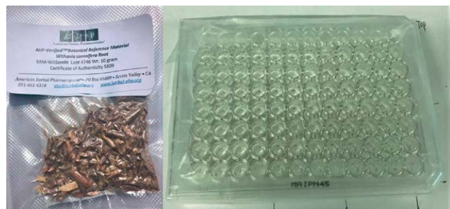
► Fig. 1 W. somnifera root certified from American Herbal Pharmacopoeia and Gentest Pre-coated PAMPA plate system.
