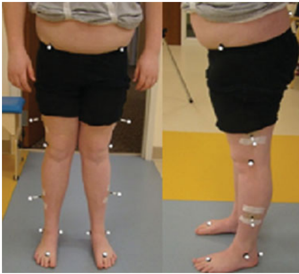
Fig. 1 Lower limb Plug-in-Gait marker set. Markers are placed bilaterally on the ASIS, PSIS, thigh, knee, shank, lateral malleolus, medial malleolus, heel, and second toe. If the ASIS markers are obstructed, they are moved 1 cm laterally. ASIS, anterior superior iliac spine; PSIS, posterior superior iliac spine.
